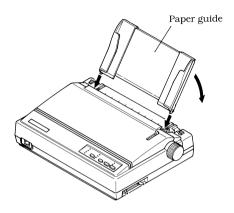
☐ To remove the paper guide from the printer, simply pull the tabs out of the holes.
